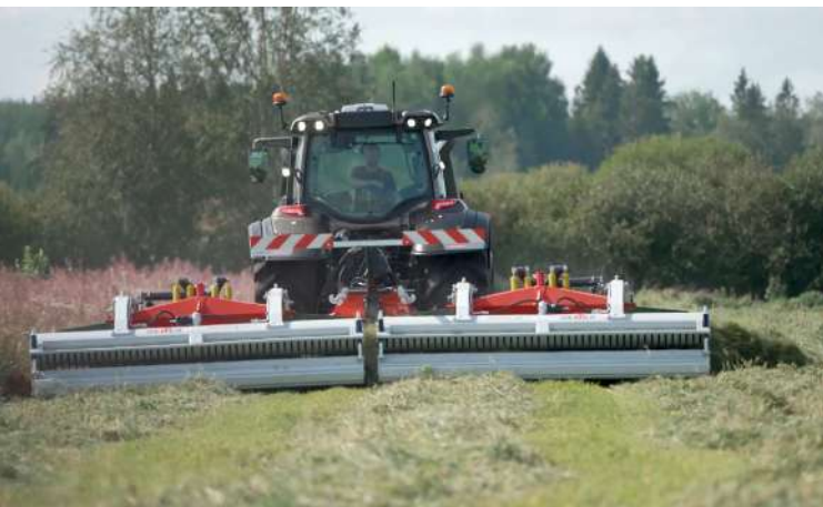
Rotor module: Suspension and damping from the rotor can be adjusted.
