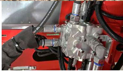
The belt valve determines the depositing direction and the belt speed - both adjustable via the terminal.
