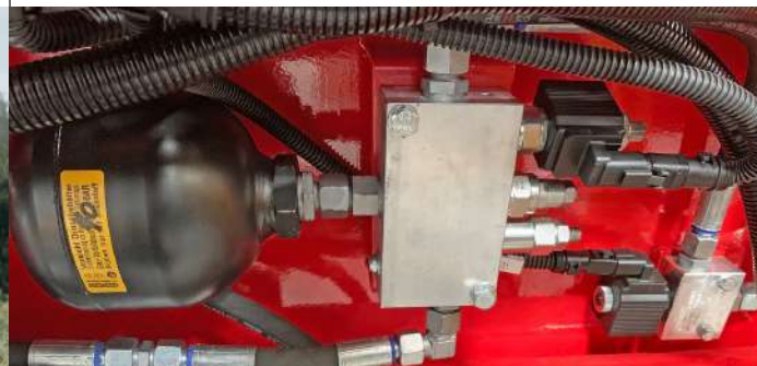
Rotor module: Suspension and damping from the rotor can be adjusted.
