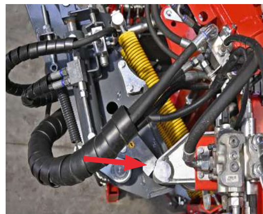
Transport securing of the working units via hydraulic spring clamp
