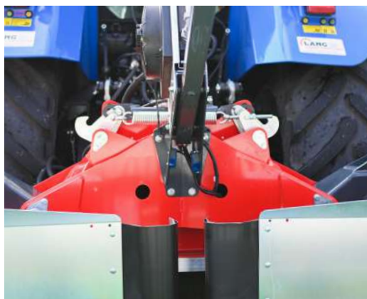
Mechanical transport lock of the outriggers
