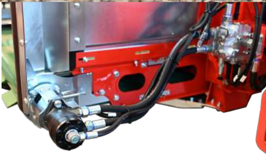
Belt drive is via hydraulic motor OMR with leakage oil line - a coupling for tension-free drive sits in between.
