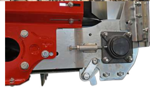
Belt roller bearing via robust standard flange bearings - adjustable scrapers clean the rollers.
