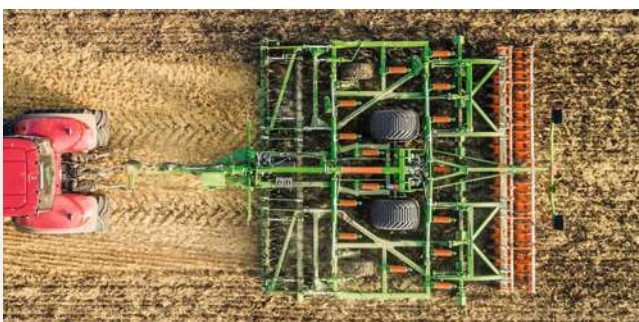
A tine for wheel track loosening runs behind each wheel
