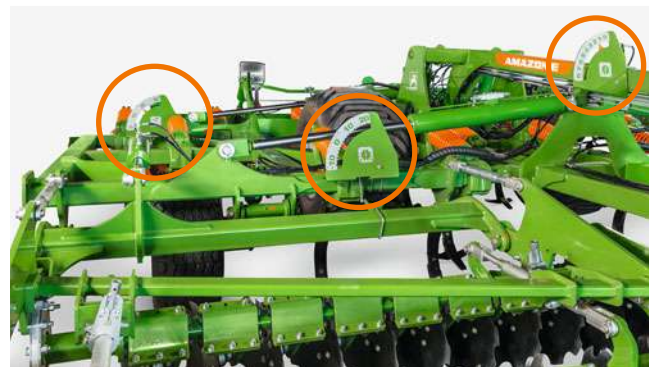
Working depth displays of the three tool elements all in one view
