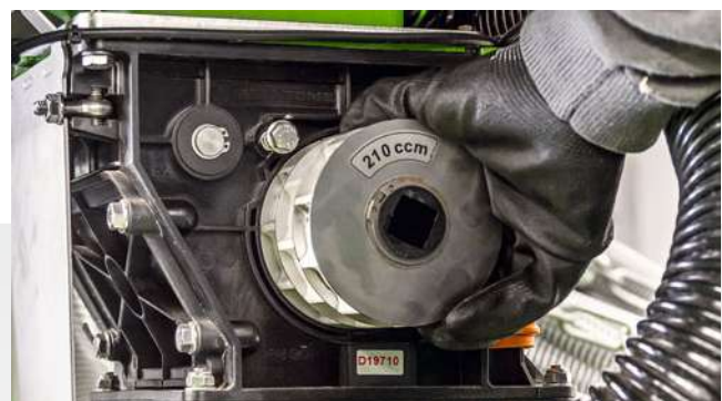
Easy exchange of the metering rollers
