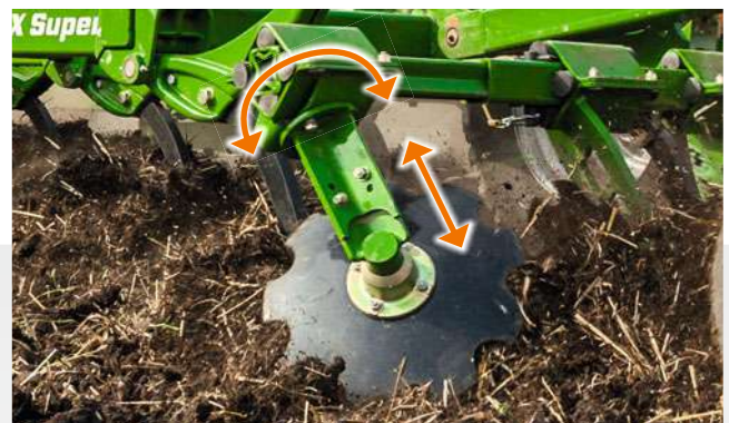
The outer closers – individually adjustable in height and angle
