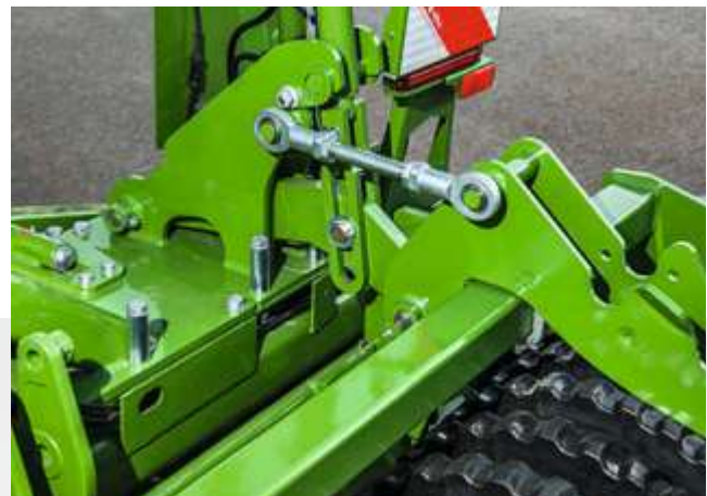
Parallel guidance of the roller
