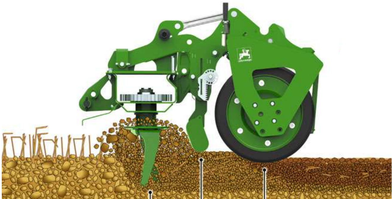
KG rotary cultivator with “on-grip” tines
