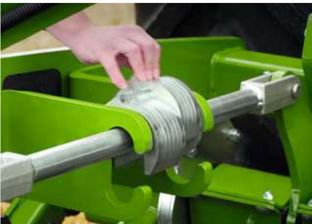
Working depth adjustment via spacers – here at a shallow working depth
