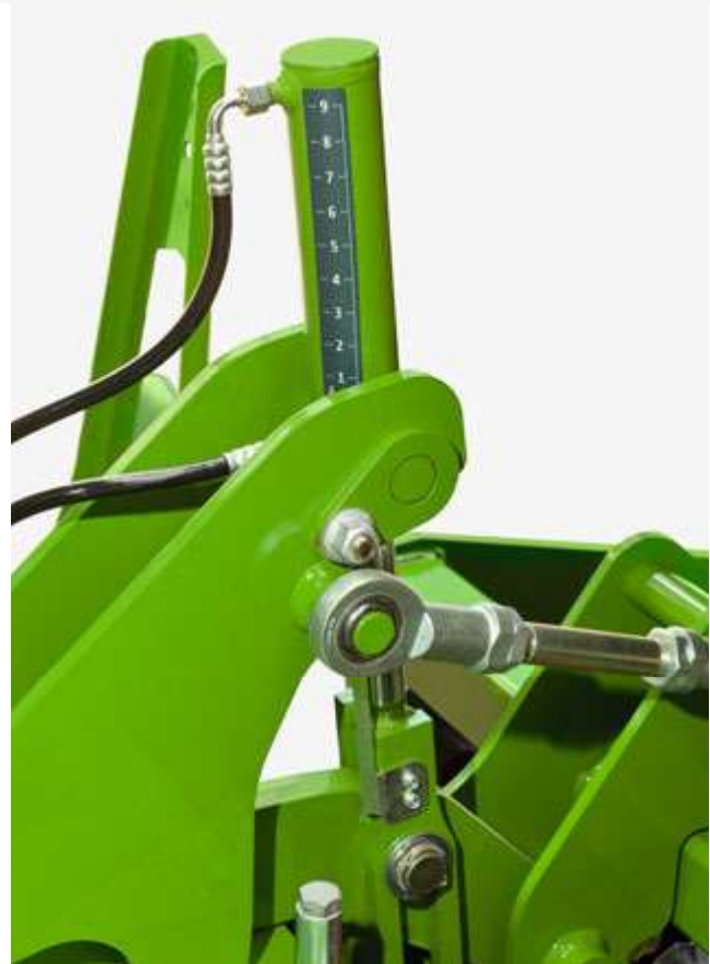
KX/KG hydraulic depth adjustment
