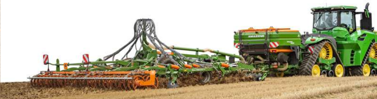
XTender 4200 mounted hopper with a capacity of 4,200 l with Ceus 7000-2TX
