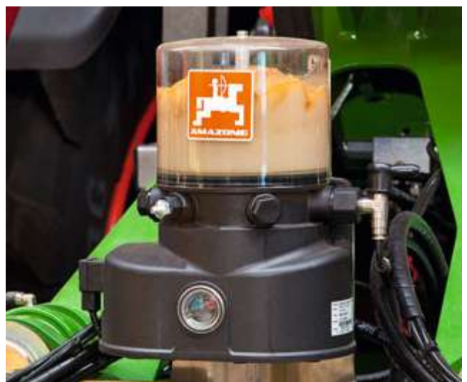
Pump with reservoir
