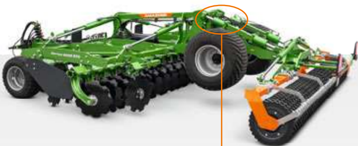
Hydraulic top tie bar on Certos 6002-2TX
