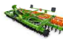
Catros mounted and trailed compact disc harrows working width 2.5 m to 6 m
