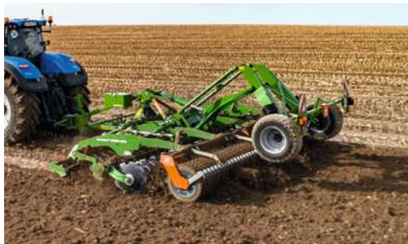
Catros XL 6003-2TS with up-front knife roller
