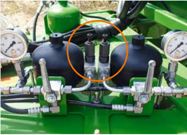
Drawbar damping system as standard
