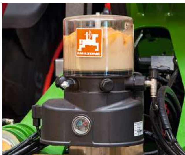
Pump with reservoir
