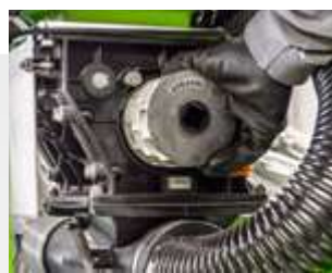
Easy exchange of the metering rollers
