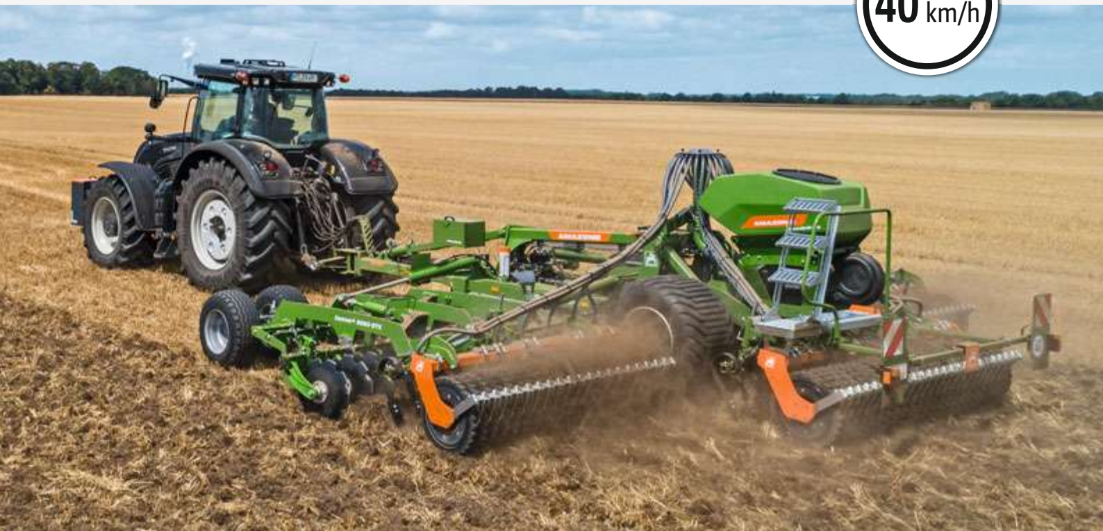
Catros XL 8003-2TX being used for stubble breaking
