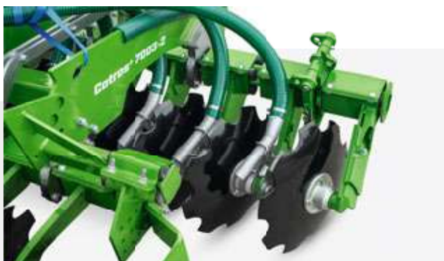
Slurry application after the first disc
