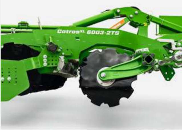
Catros XL 6003-2TS at the minimum disc depth The discs are completely swivelled in towards the frame
