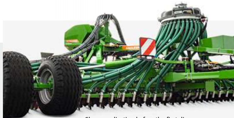
Slurry application before the first disc
