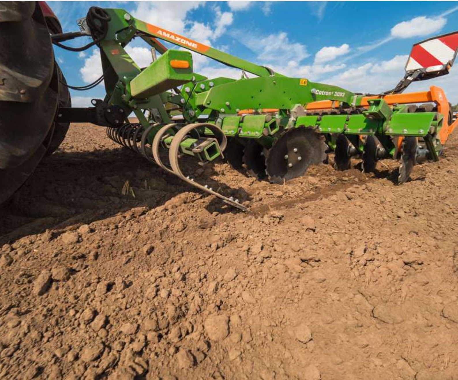
Catros + 3003 in operation with the Crushboard
