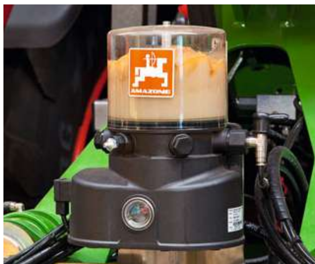
Pump with reservoir
