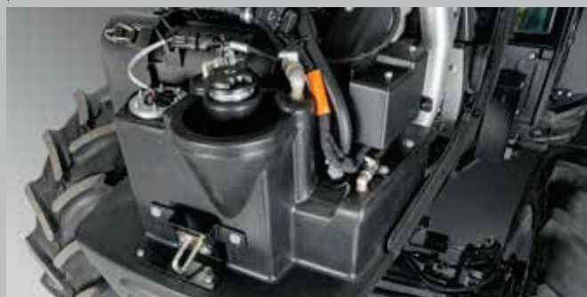
The fuel tank built into the front axle block can be filled with the hood closed, while an additional tank is located below the chassis.
