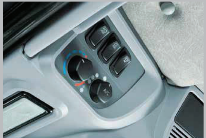
The air conditioning and working headlight controls are easy to reach in the roof.
