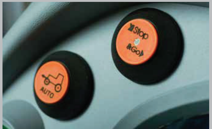
Stop&Go. Start and stop the vehicle in comfort without using the clutch pedal.
