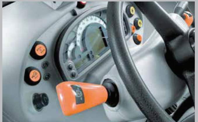
Power shuttle. Change the direction of travel with a single touch.
