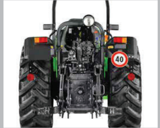
3 Standard Hydraulic Remotes make the 80F the perfect match for almost any application.
