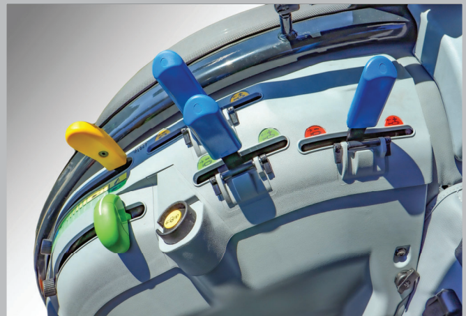
Controls for the rear power lift and hydraulic working equipment: close together and easy to access.
