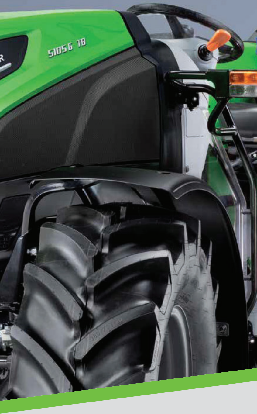
Front axle: 50-degree steering angle; electro-hydraulic 4wd; integrated front axle brakes; fully locking differential.
