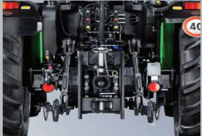
The rear 3-point hitch: up to 7,900 lb (4,525 kg) lifting capacity, extremely precise control. 540/540E rear PTO as standard.
