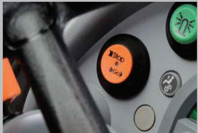
Stop&Go system: stop and start the tractor using only the brake pedal.
